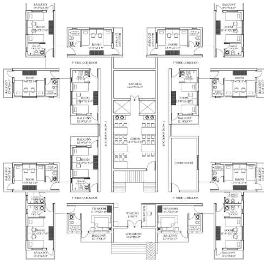
GROUND FLOOR PLAN Built-up area = 7645 Sq.Ft.
